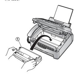
**12** Close the front cover (①) by pushing down on both sides, until locked.
